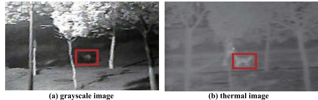
Fig. 1. An example of grayscale-thermal video pairs. The grayscale video sequence has very limited illumination, while the thermal video sequence is robust to the illumination changes. Grayscale-thermal tracking aims to exploit the complementarity property to guarantee the robust tracking performance in both thermal and grayscale sequences.
