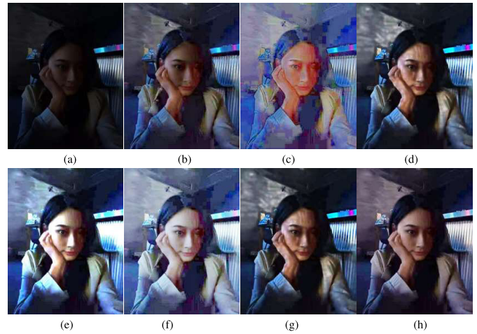
Fig. 2. Image enhancement results of a real-world low-light example. (a) Input low-light image, and the enhancement results of (b) LIME [7], (c) RetinexNet [10], (d) SSIENet [16], (e) RUAS [17], (f) Zero-DCE++ [18], (g) SCL-LLE [19], and (h) our Low-FaceNet. By leveraging facial semantics and low-light images, which are often ignored in previous approaches, our Low-FaceNet achieves results that are not only brighter but also more visually appealing.
