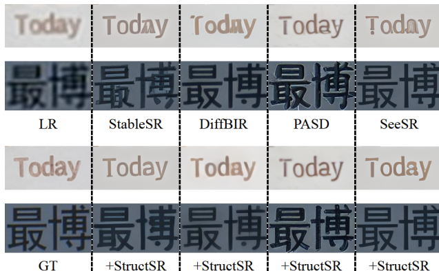
Figure 1: Comparison of diffusion-based Real-ISR methods with and without StructSR integration. The original methods generate spurious details in both English letters and Chinese characters. Integration with StructSR significantly reduces these artifacts, resulting in more accurate reconstruction.
