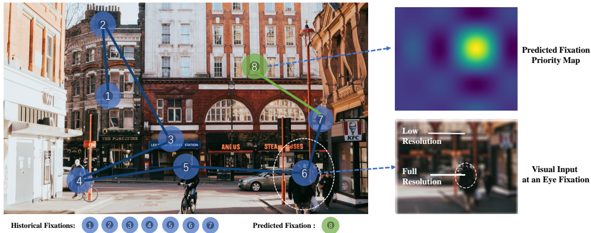
Figure 1: Human scanpaths are composed of a series of fixations and saccades. Visual inputs at the fovea are processed in high resolution during fixations, while peripheral vision is correspondingly blurred to guide saccades. A scanpath prediction model simulates human saccadic decisions by predicting the priority probability map of the next fixation.
